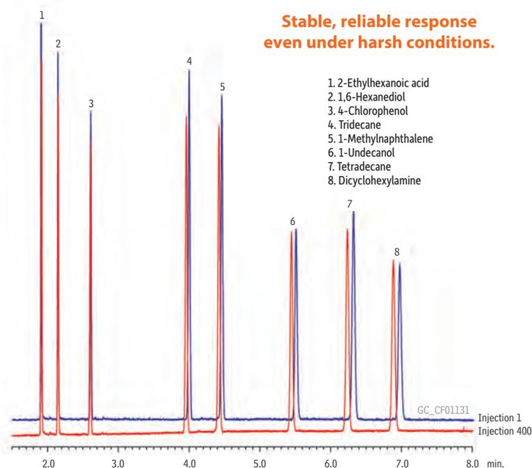
**Column:** Rxi<sup>®</sup>-5Sil MS, 30 m, 0.25 mm ID, 0.25  $\mu$ m (cat.# 13623); **Sample:** Column test mix (cat.# 35226); **Inj.:** 1.0  $\mu$ L split (split ratio 1:60), 4 mm recessed single taper (cat.# 20983); **Inj. temp.:** 250  $^{\circ}$ C; **Carrier gas:** helium, constant pressure; **Linear velocity:** 36 cm/sec @ 125  $^{\circ}$ C; **Oven temp.:** 125  $^{\circ}$ C; **Det:** FID @ 320  $^{\circ}$ C; **Instrument:** Agilent 6890
