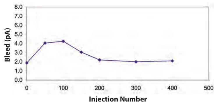
Column bleed over 400 injections of HFBA derivatization reagent. Column was held at the maximum isothermal temperature.
